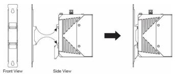
There are two options for installation: The first option is to hook the EDS DIN-rail latch on the opening of the wall mount kit (see picture above) and then mount the wall-mount kit on the wall with screws. (The other option is to perform these two steps in the other order.) The heads of the screws should be less than 6.0 mm in diameter, and the shafts should be less than 3.5 mm in diameter, as shown in the figure at the right.
