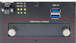
**Step 2:** Slide the latch on the disk tray to the left and pull out the tray from the slot.
