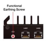
**NOTE** A 4 mm² conductor must be used when the connection to the external grounding screw is utilized. The heat sink is grounded to the chassis by an internal screw.
