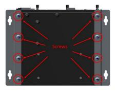
**STEP 2**: Use two screws ( $\emptyset$ 3.7 mm, 60 mm in length) per side to attach the MC-7400 to a wall or cabinet.
