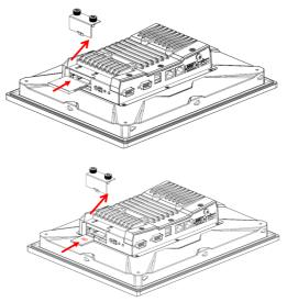
3. Reattach the cover and secure it with screws.
