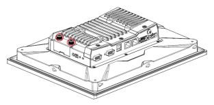
2. Insert the CFast or SD card into the slot using the push-push mechanism.
